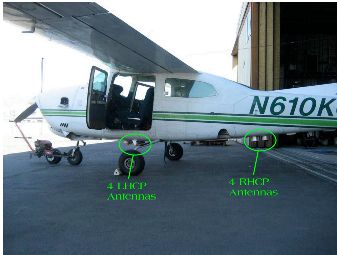
: 4 LHCP and 4 RHCP antennas installed on the aircraft
