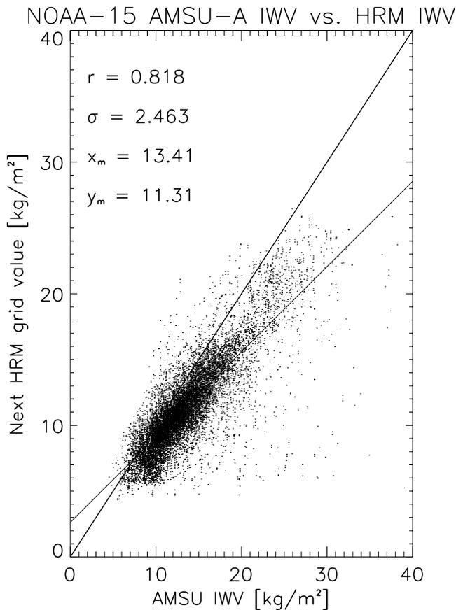
Fig. 3. Integrated water vapor (IWV) derived from AMSU-A data of NOAA 15 between 26th and 30th of April 2001 over the sea within the BALTEX area compared with the IWV of the HRM model.  $r$  is the correlation coefficient,  $\sigma$  is the standard deviation of the difference (HRM-AMSU),  $x_m$  is the mean value of the AMSU IWV,  $y_m$  is the mean value of the HRM IWV. The 1:1 line as well as a linear fit are given.
