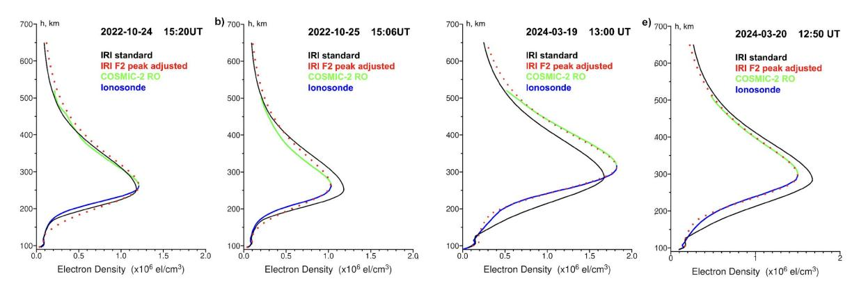
Comparison of the IRI-2020 adjusted EDPs (red dots) with reference combined EDPs (blue-green line). The standard IRI output is shown as a black line.
