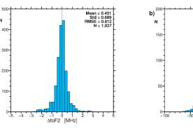
Histograms of the F2 peak parameters residuals  $\Delta \text{foF2}$  ( $\Delta \text{foF2} = \text{foF2}_{RO} - \text{foF2}_{ionosonde}$ ) and  $\Delta \text{hmF2}$  ( $\Delta \text{hmF2} = \text{hmF2}_{RO} - \text{hmF2}_{ionosonde}$ ) between collocated COSMIC-2 and ionosonde measurements
