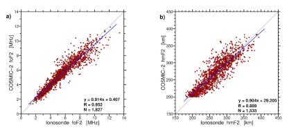
The scatter plots of the COSMIC-2 RO-based foF2 and hmF2 values against the corresponding ionosonde-derived ones.
